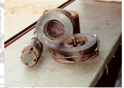
Cavitation damage on boiler feedwater pump minimum recirculation valve trim.
